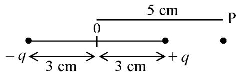
The electric potential (in  $10^2 \text{ V}$ ) at point P due to the dipole is ( $\epsilon_0$  = permittivity of free space and  $\frac{1}{4\pi\epsilon_0} = K$ ):
